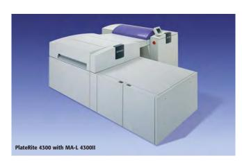
hold up to 100 plates and automatically removes interleaf paper before loading each plate. It is also possible to upgrade from the SA-L 4300II to the MA-L 4300II multi-cassette autoloader, which comes standard with three cassettes and enables up to 300 plates of three different sizes to be loaded and imaged in the PlateRite 4300S without operator intervention. The PlateRite 4300S and PlateRite 4300E can also be paired with the more economical SA-L 4100\* single-cassette autoloader.
