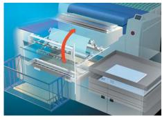
The arm goes to pick up the plate, and the plate is hoisted up to the engine section.
