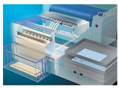
3 The interleaf paper is lifted away and ejected into an external collection box.
